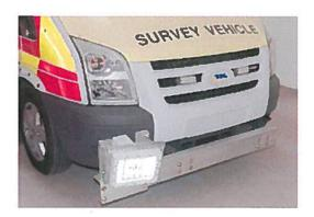
Road markings are an important safety element on our highways. TRL has developed the MarkingCollector, a technology that measures with pinpoint accuracy the condition of the markings from a vehicle travelling with the normal traffic flow.
