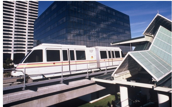
Automated guideway transit trains provide distributor or shuttle service without an on-board operator, offering the potential for lower operating costs. The Jacksonville Transportation Authority Skyway provides service within downtown Jacksonville and to stations across the St. John's River. Automated guideway transit modal data are included with other rail modes in Tables 35 and 39.
