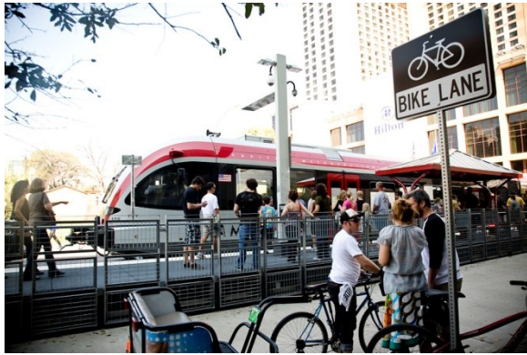
Hybrid rail provides commuter rail-type service using light-rail-type vehicles. Capital Metro hybrid rail trains operate from downtown Austin, TX, to distant northern suburbs. Hybrid rail data are reported in Tables 35 and 36.
