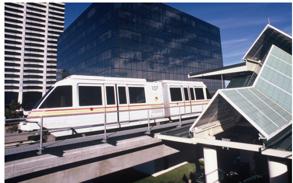
Automated Guideway Transit trains provide distributor or shuttle service without an on-board operator, offering the potential for lower operating costs. The Jacksonville Transportation Authority Skyway provides service within downtown Jacksonville and to stations across the St. John's River. Automated Guideway Transit modal data are included with other rail modes on on Tables 35 and 39.
