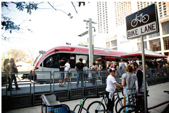
Hybrid Rail provides commuter rail-type service using light rail-type vehicles. Capital Metro Hybrid Rail trains operate from downtown Austin, TX, to distant northern suburbs. Hybrid Rail data are reported on Tables 35 and 36.
