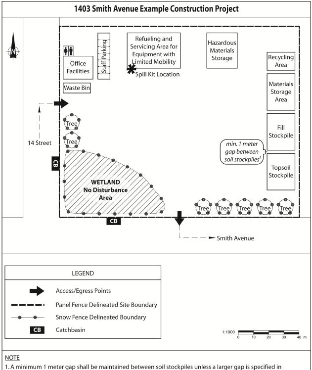
1. A minimum 1 meter gap shall be maintained between soil stockpiles unless a larger gap is specified in legislation that applies to your site.
