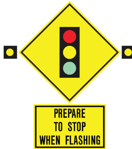
Figure 18 – Active Advance Warning Beacon
