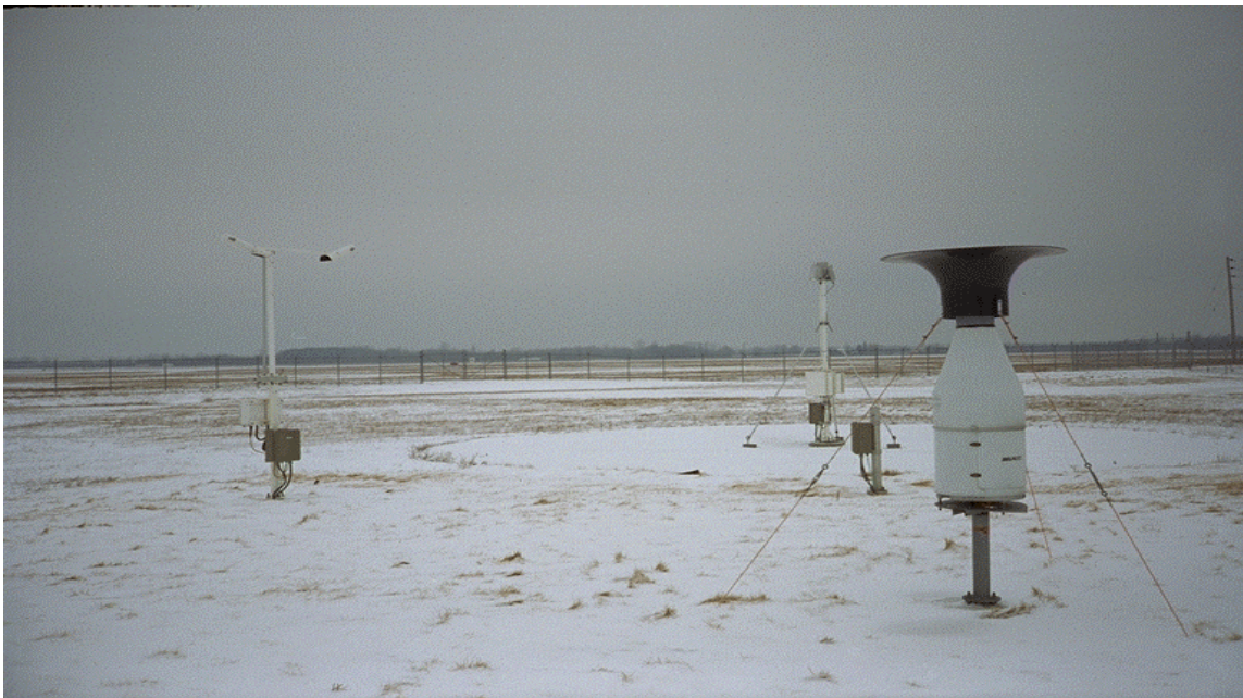
Photo 2.14 Meteorological Services Canada's Automated Weather Station Instruments
