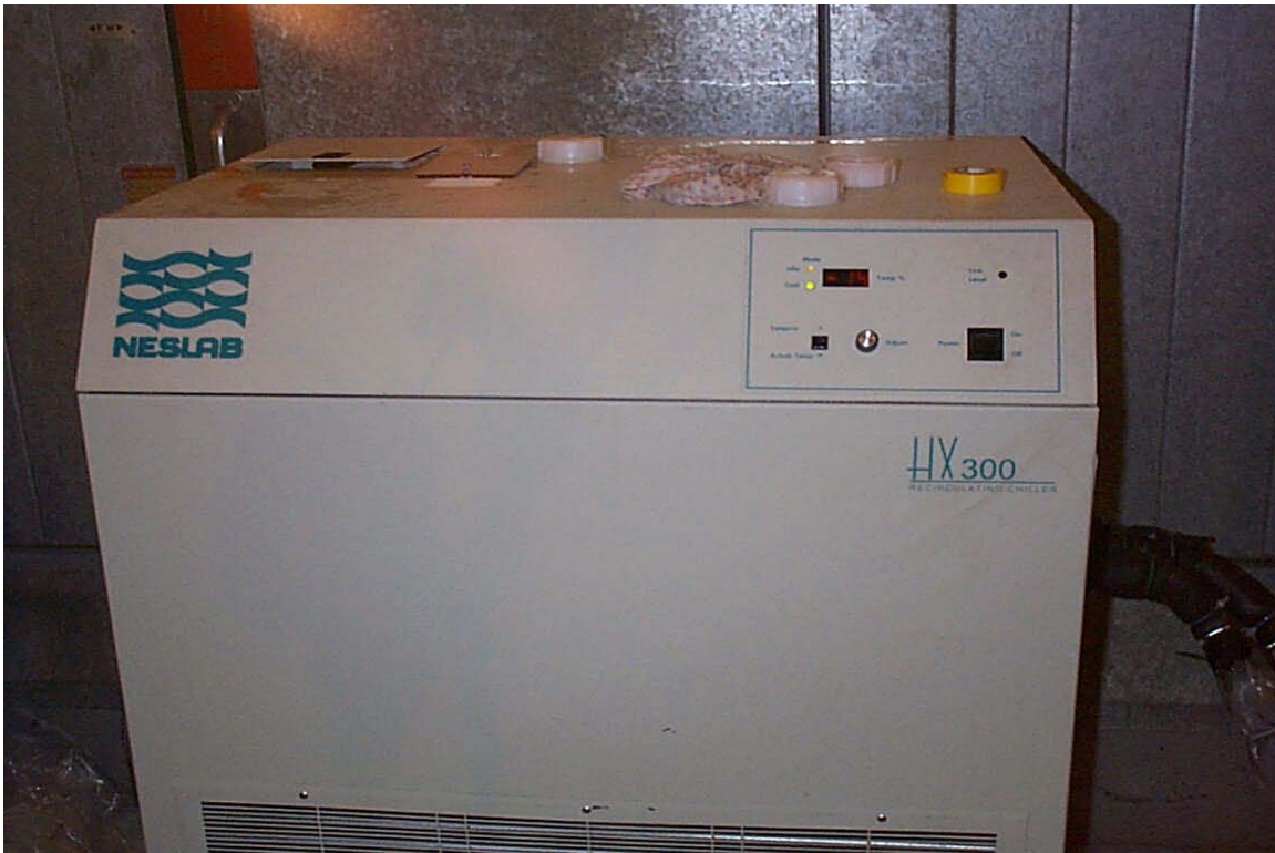
Photo 2.13 New Cooling Unit for Cold-Soak Boxes
