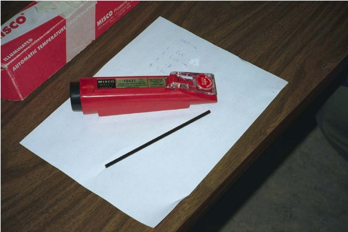
Photo 2.15 Misco Refractometer Used to Measure Freeze Point
