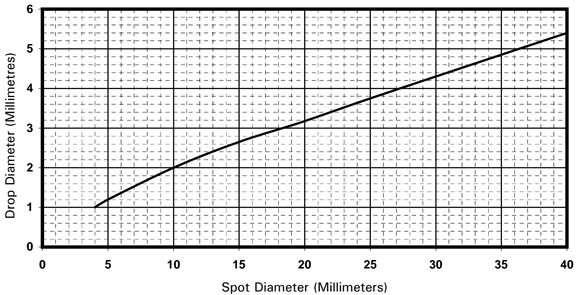
FIGURE 2.3 CONVERSION OF SPOT DIAMETER TO DROP DIAMETER WHATMAN # 1 FILTER PAPER
