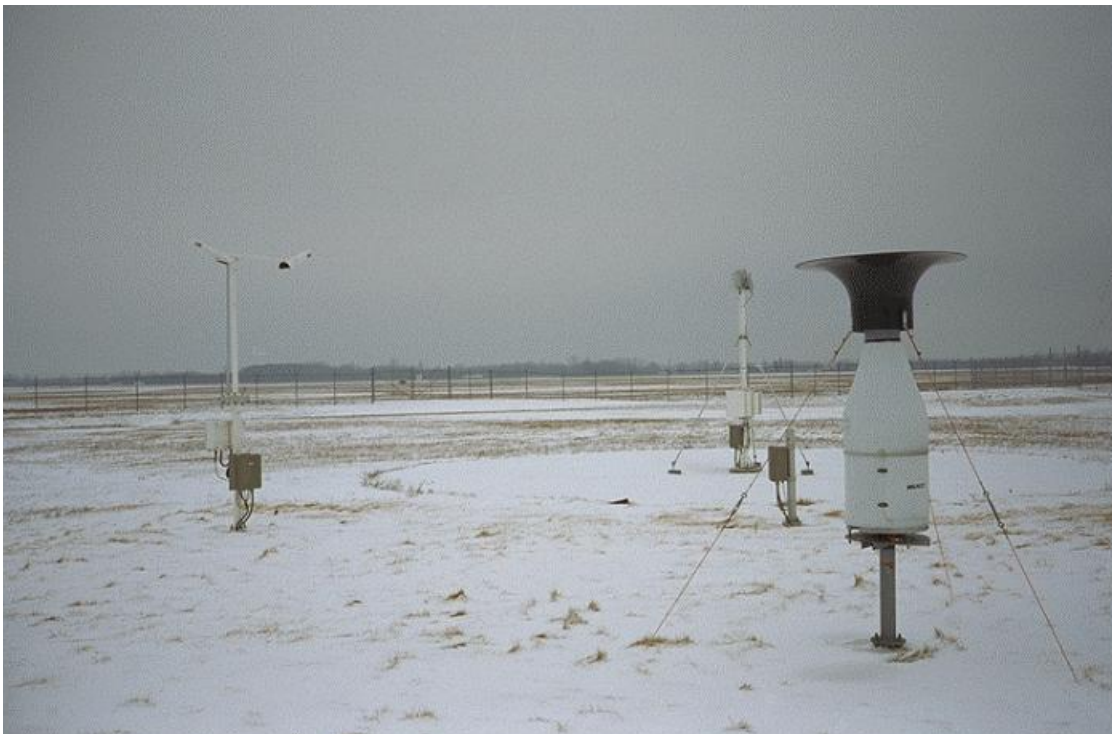
Photo 2.16 Atmospheric Environment Services Automated Weather Station Instruments
