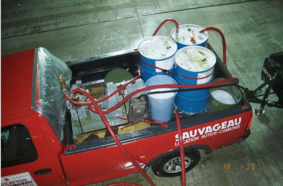
Photo 6.5 Mobile Type IV Sprayer
