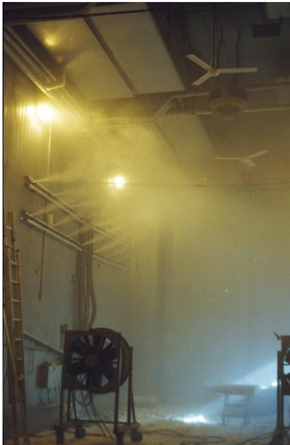
Photo 6.2 Snow Spray Bar in Operation
