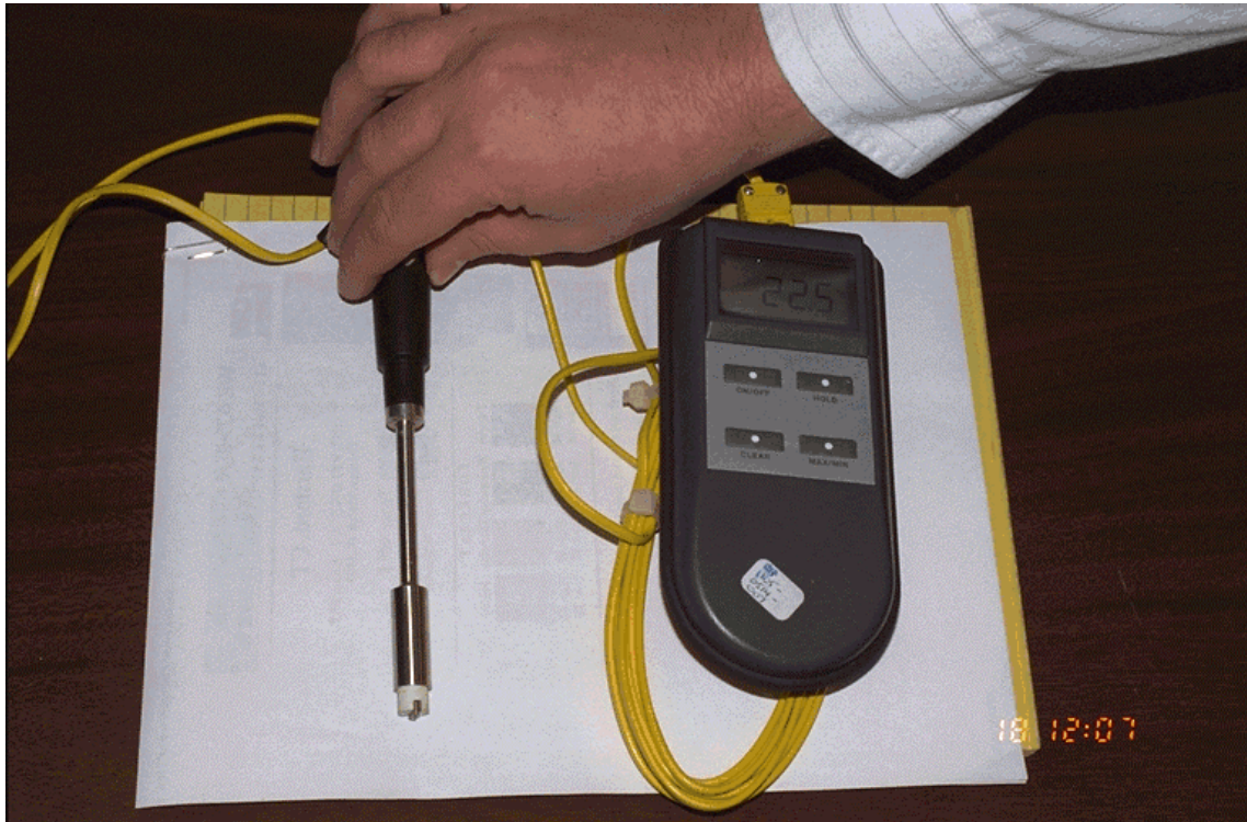
Photo 2.17 Hand-held Temperature Probe
