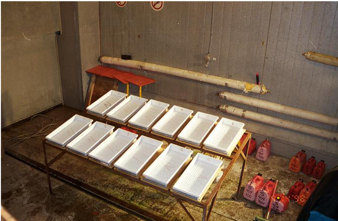
Photo 2.11 Collection Pans Used Indoors at the NRC
