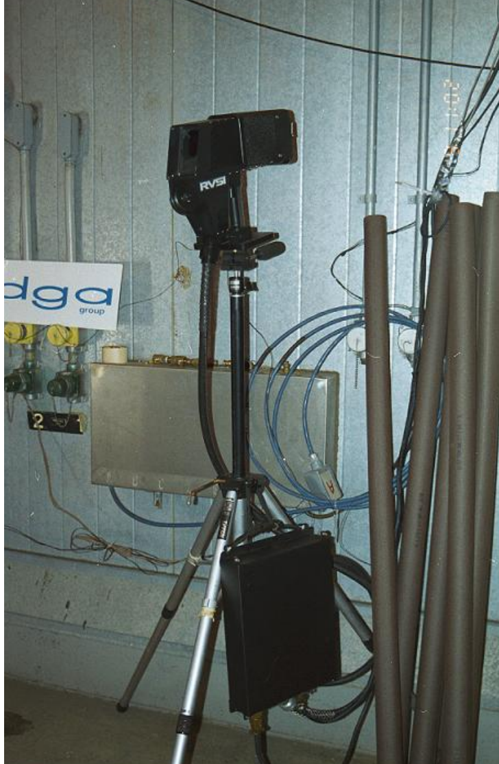
Photo 2.14 Hand-held RVSI Ice Detection Unit
