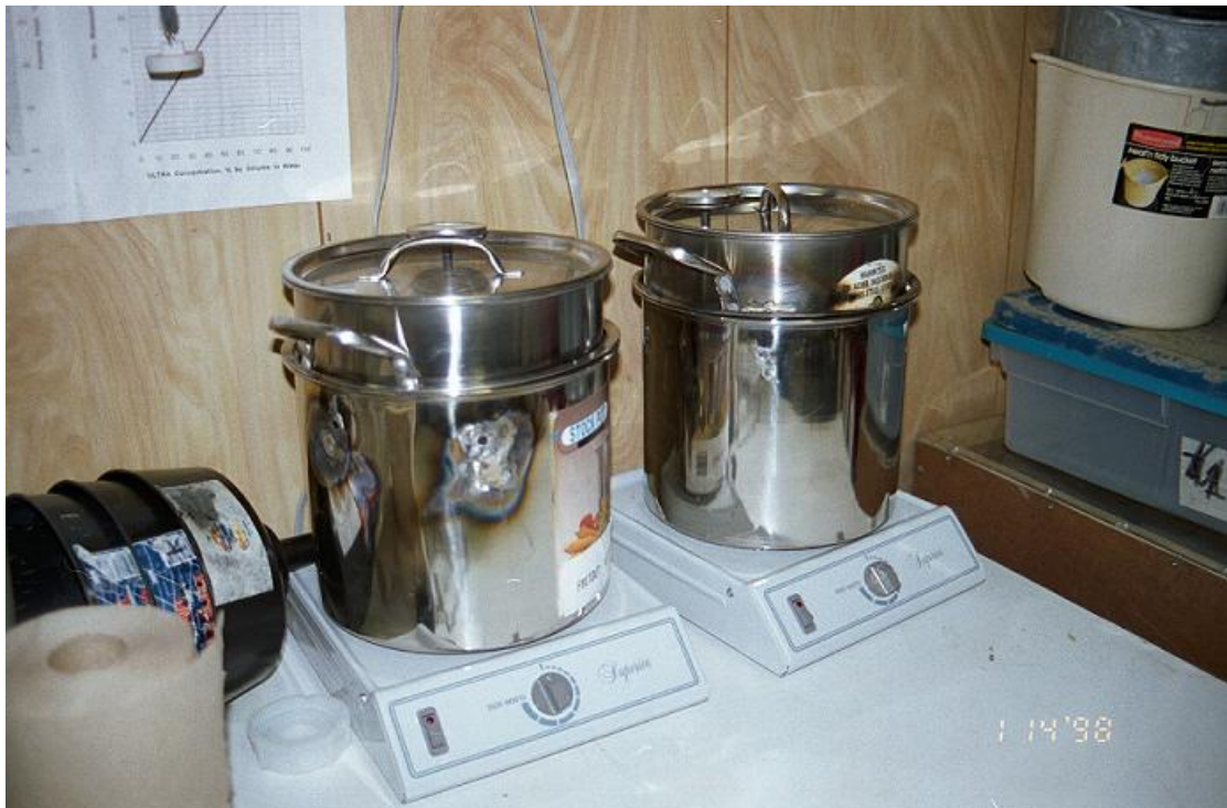
Photo 4.2 Double-Boiler System Used for Heating Type IV Fluid to 80°C
