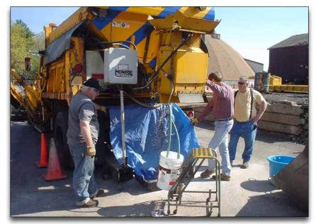
Open Loop ground speed controllers are the next most accurate method of controlling discharge/application rate. The controller senses the ground speed of the spreading vehicle from the speedometer or other sensing point, and changes product delivery rate in proportion to vehicle speed.
