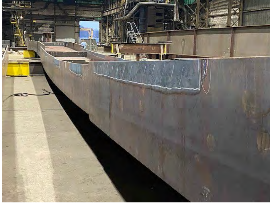
Figure 51. Photo. Horizontal heat curving with strip heats.
