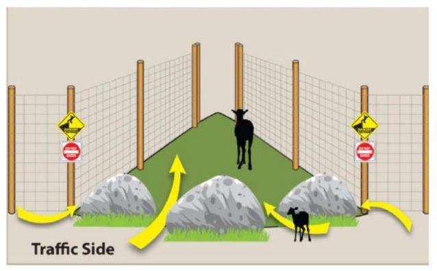
Figure 7. Open escape gate with wing fencing [39]
