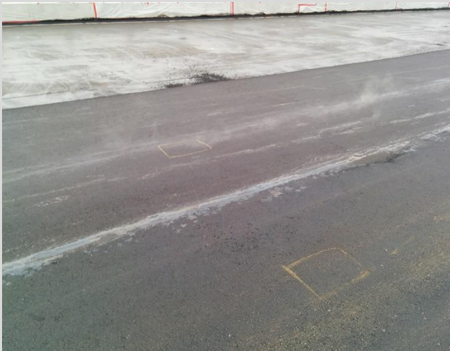
17.7 Control strip method used to determine maximum density. Location for nuclear densometer marked for consistent testing.
