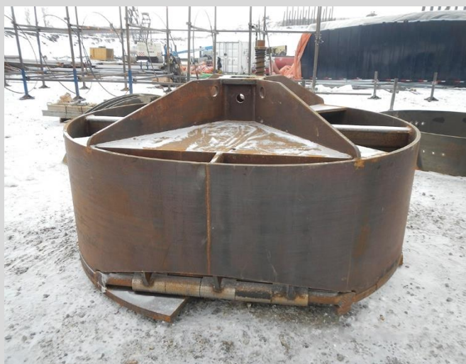
3.17 Large muck or slush bucket, used to clean out the bottom of wet or muddy holes prior to cage placement.
