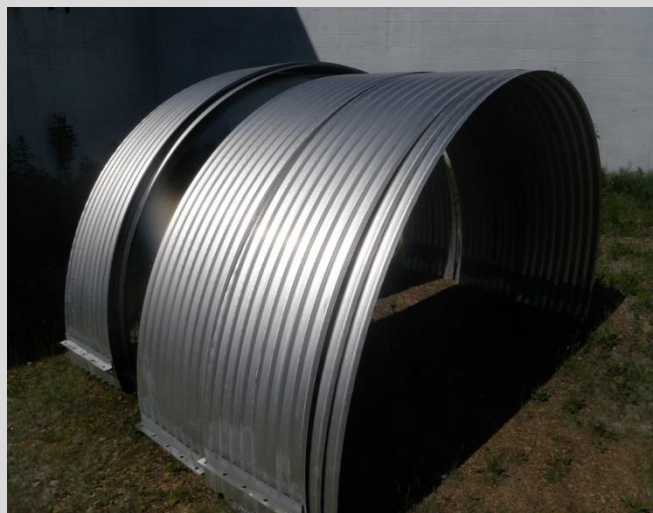
18.12 Storage of CSP couplers in concave down position to prevent storage staining.
