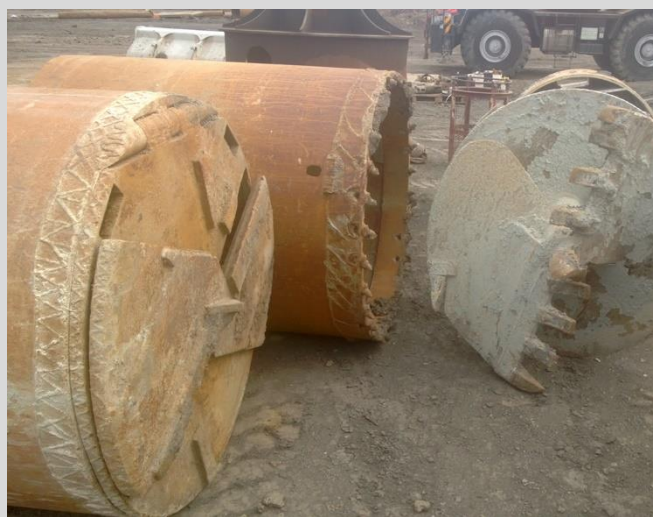
3.14 Slush bucket, coring barrel and augers shown.
