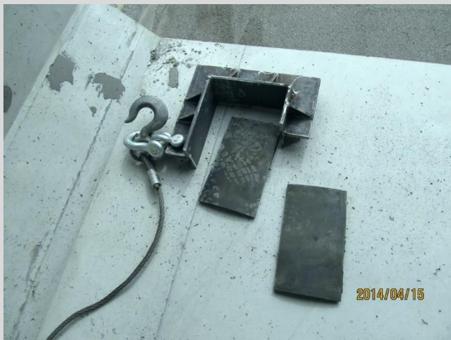
26.19 Typical Winching bracket hardware.
