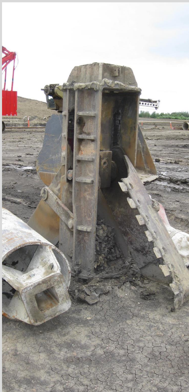
3.19 Belling tool, fully opened. Wings are opened at the tip elevation to create a belled pile.
