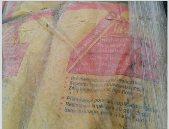
7.39 Approved grout product stored on site. Expiration dates need to be labelled on package.
