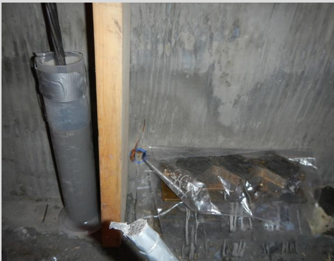
7.38 Modified bleed test with graduated cylinder on left. Grout cubes for compressive strength testing cast in brass mould.
