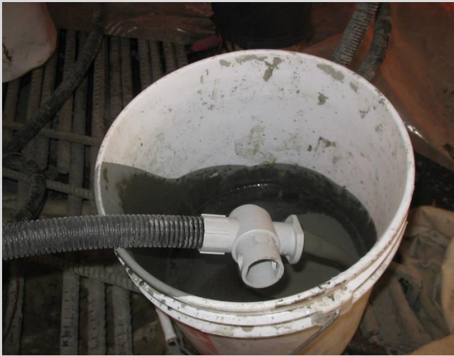
7.36 Grout sampled for testing.
