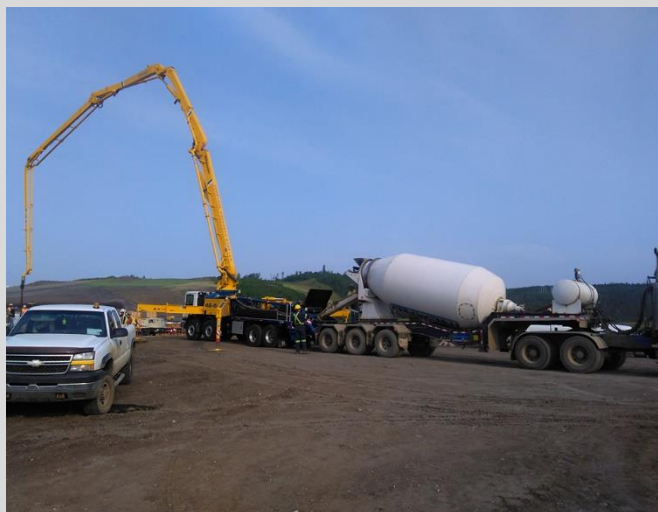
4.105 Typical trailer-type concrete mixer and concrete pump.
