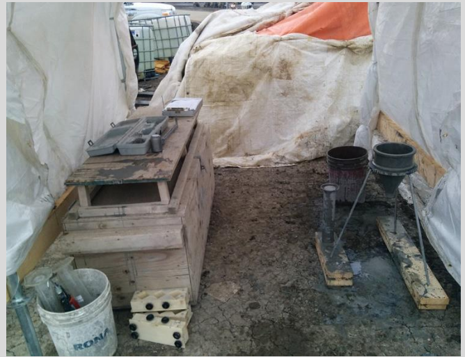
7.37 Grout testing equipment. Efflux test performed with flow cone, modified bleed test with graduated cylinder and mud balance used to determine density. Grout cubes cast for compressive strength.
