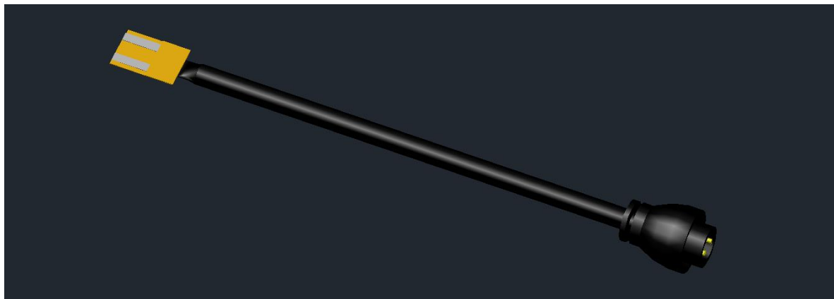
Figure 4.2 AutoCAD drawing for the Ice state and Presence Sensor Sensing Element and Connector.
