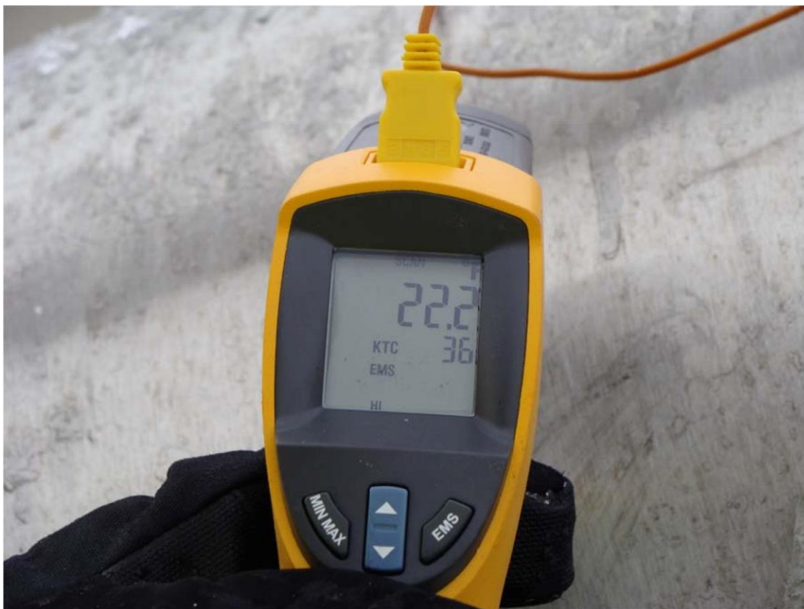
Figure 1.13: Thermocouple reading between ice and stay February 23, 2011
