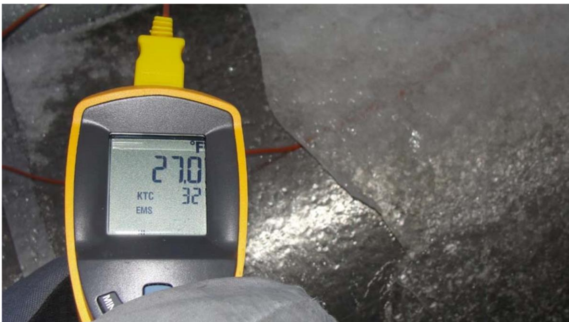
Figure 1.14: Thermocouple reading between the ice and stay February 24, 2011
