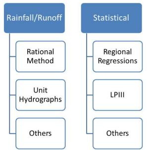
Figure 3.3. Hydrologic model types and examples.
