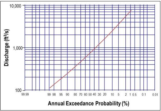
Figure 3.4. Example of a flood frequency curve.
