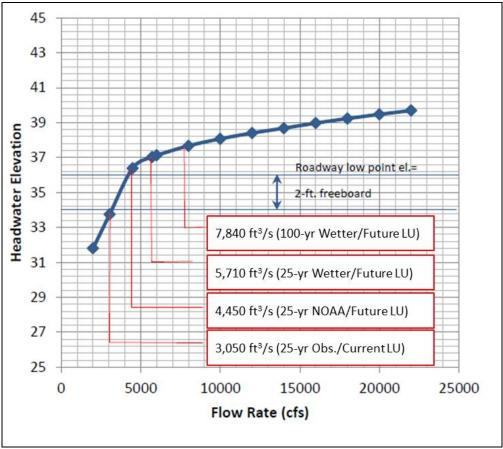
Figure 8.5. Performance curve for existing Airport Boulevard culvert.
