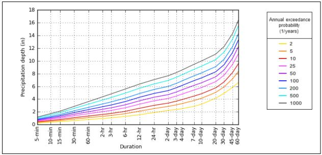
Figure 7.1. Depth-duration-frequency curve from NOAA Atlas 14.
