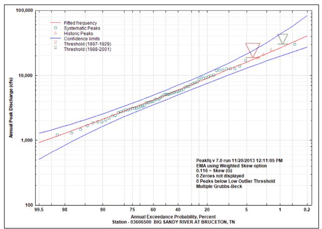
Figure 3.5. Example flood frequency curve with confidence intervals.
