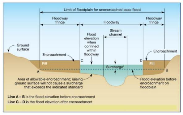
Figure 2.2. Example floodplain cross-section.
