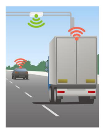
Projects in the earlier stages of research tend to focus on development of novel technologies. For example, the Active Barrier project developed a system to detect and communicate impact with guardrails, while the SARTRE project investigated road trains/vehicle platooning technology, which has the potential to transform motorway driving.
