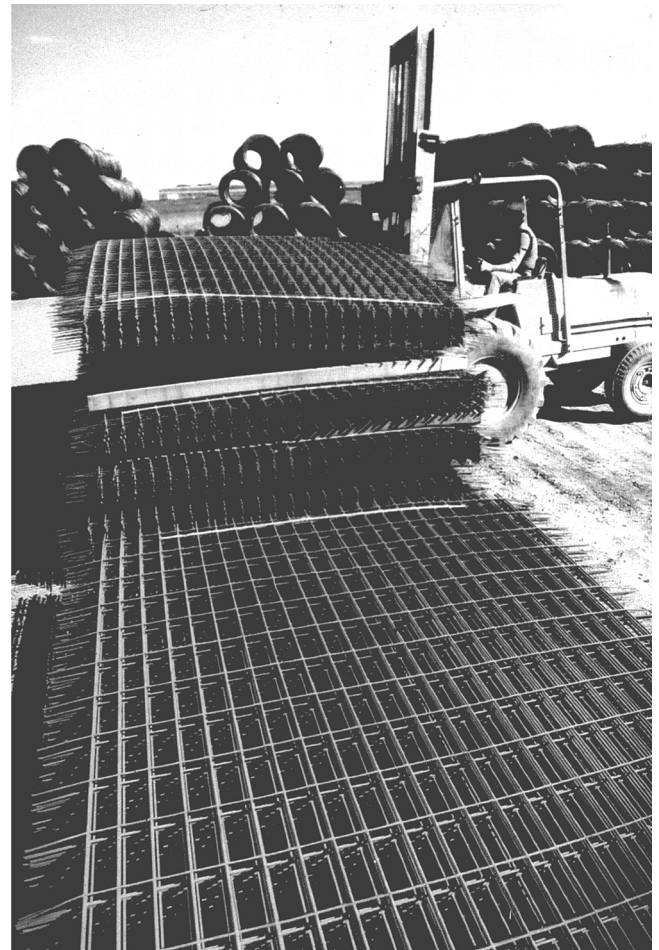
Fig. 3.1.3—Welded wire reinforcement sheets (courtesy of Wire Reinforcement Institute).
