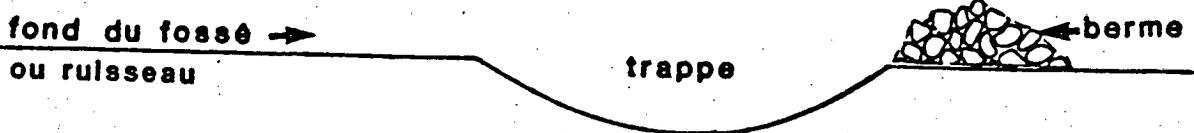
**FIGURE A-4 BERME FILTRANTE ET TRAPPE A SÉDIMENTS**
