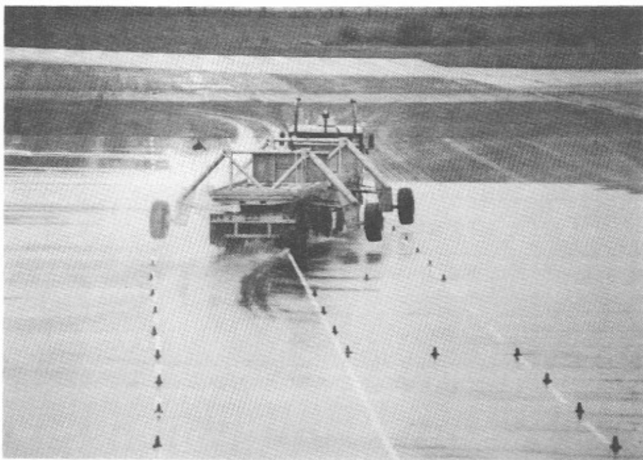
Figure 16/ Vehicle Making Evasive Manoeuvre on Low-Friction Surface
