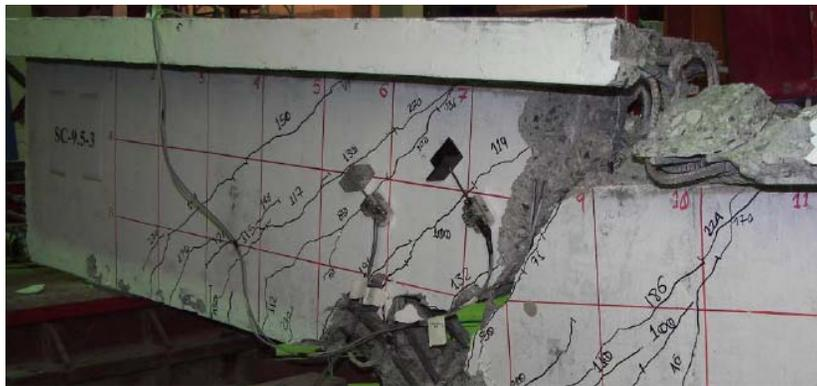
d) Poutre SC-9.5-3 – Rupture [6]
