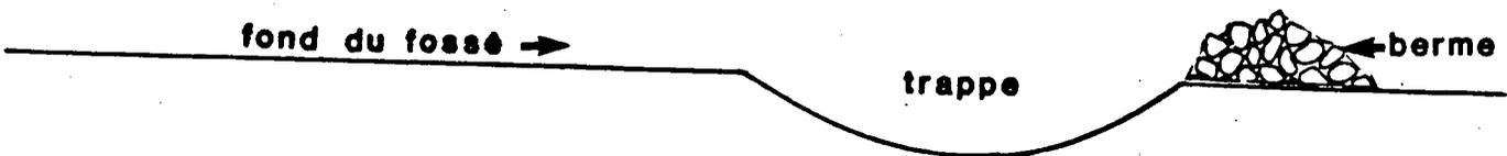
**FIGURE- 7 BERME FILTRANTE ET TRAPPE A SÉDIMENTS
