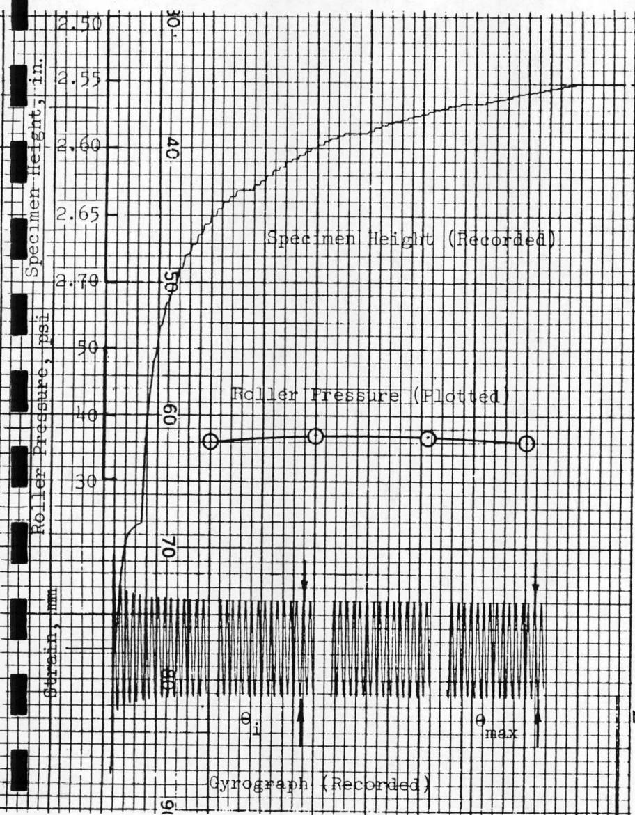
NOTE: Specimen height curve is becoming asymptotic, indicating approximate compaction equilibrium. Since roller pressure and gyrograph indicate a stable mix the vertical strain  $\epsilon$  should be largely recoverable.
