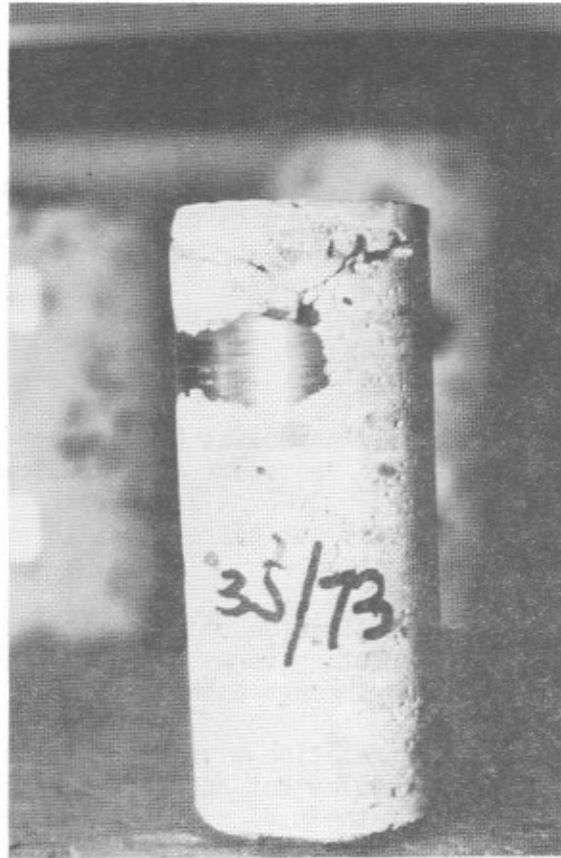
Figure 1/ Corrosion-Induced Delamination in a Concrete Core
