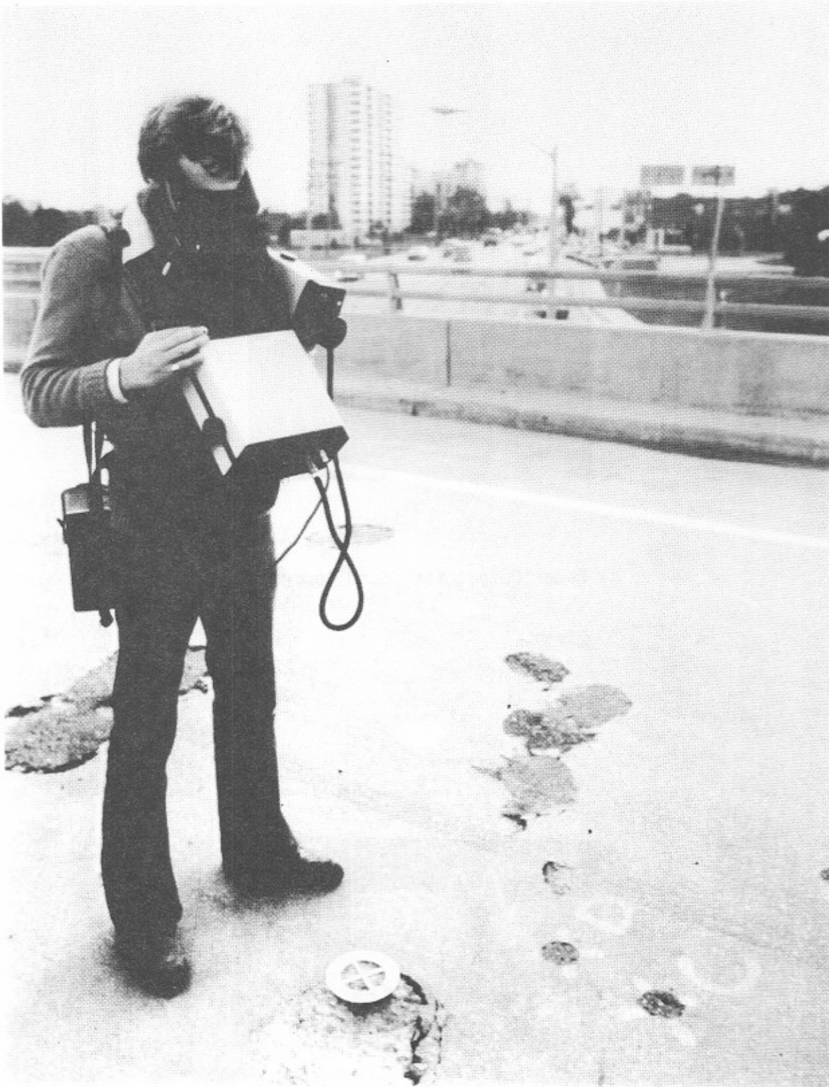
Figure 4/ Infrared Thermovision Equipment Being Operated at Ground Level]
