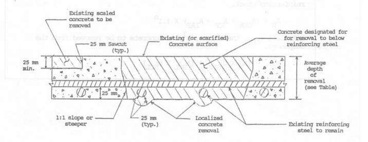
Figure 1 - CONCRETE REMOVAL DETAIL
