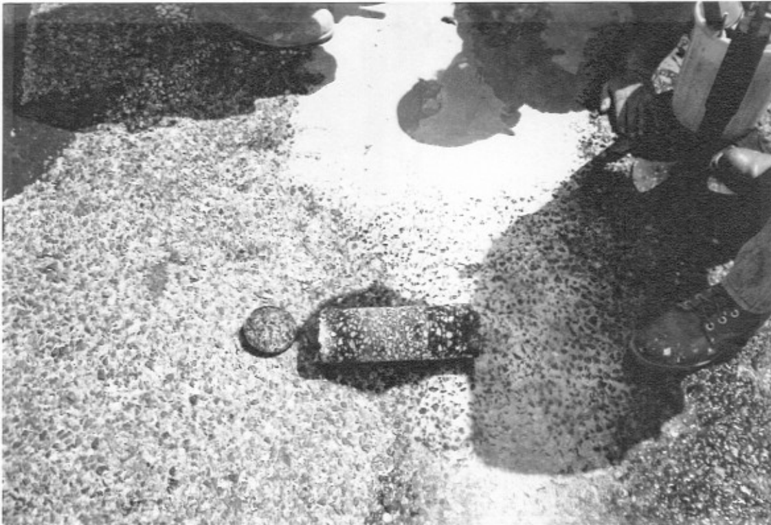
Fig. 15(a)-(b): (a) Photograph of core sample #1 taken at 1 m from the west curb and 8.6 m from the north end joint. (b) Photograph of core sample #2 taken at 2 m from the west curb and 18.75 m from the north end joint.
