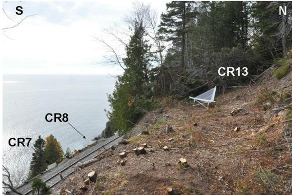
Figure 4. Trihedral or corner reflector (CR13) installed in zone I upslope of the railway.
