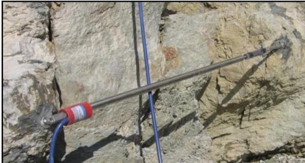
Figure 3. Crack meter (shown before installation was completed).
