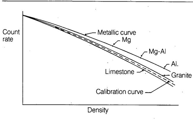
This curve corresponds to 50% granite and 50% limestone according to the procedure adopted for processing data. These two calibration blocks were chosen because most construction materials have attenuation coefficients situated within the absorption coefficients or the stopping power of these blocks.
