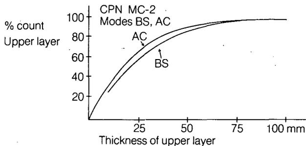
Table VIII shows the proportion of the count taken on the test material which must be considered, according to its thickness.
