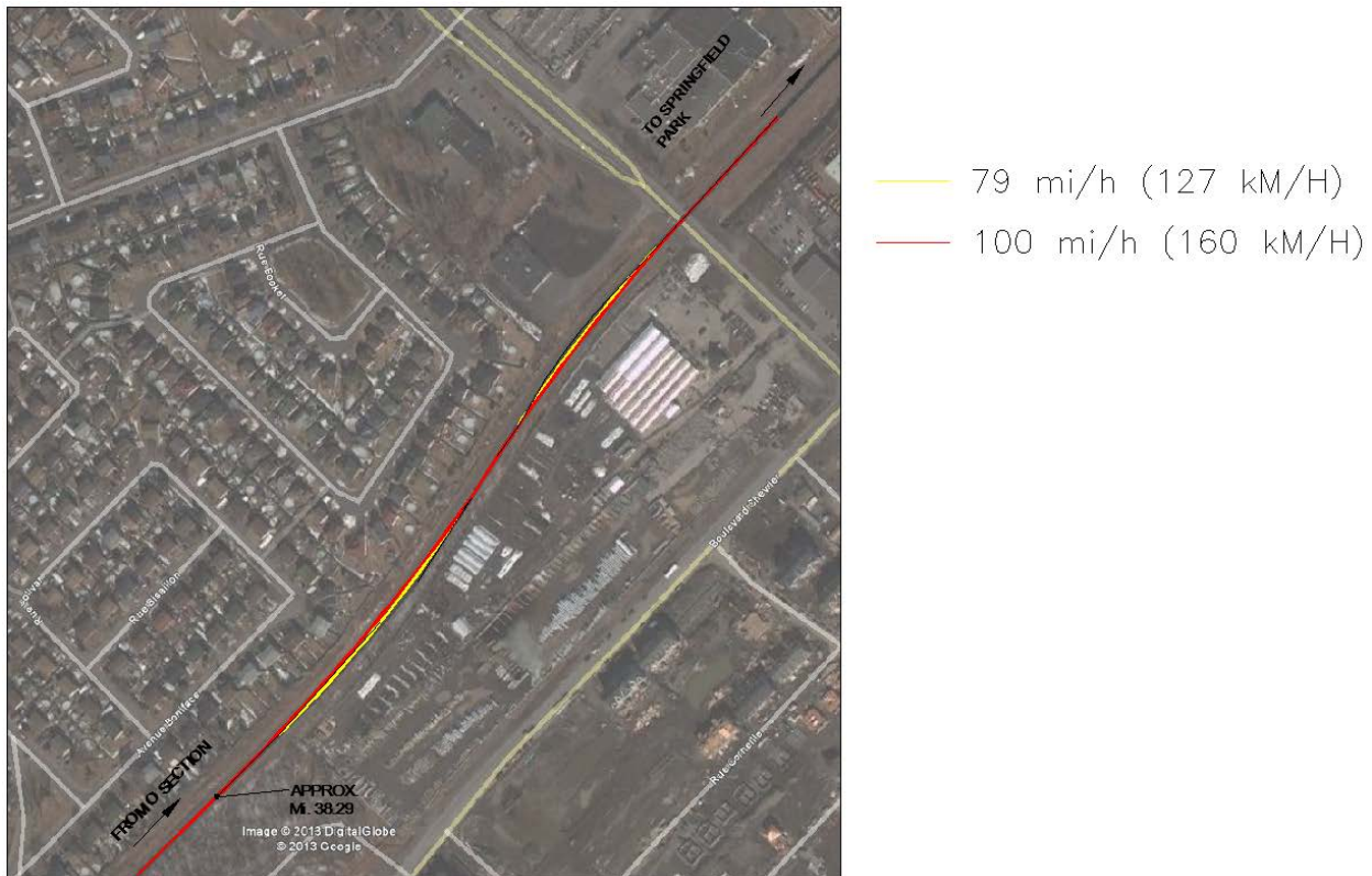
Figure 77 – Reconfiguration de la courbe – Rouses Point P.M. 38,47 – 38,59
