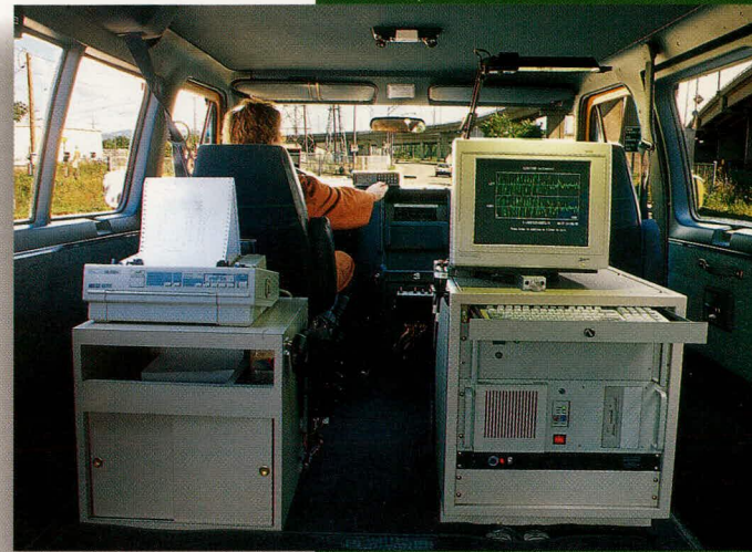
The inertia profilometer takes precision measurements which are used to assess pavement profile and the application of roughness clauses in documents authorizing road construction. (Photo: Jacques Lessard)
