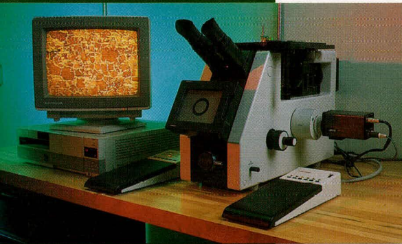
The metallograph is a video optical device used to examine the internal structure of metals. It is indispensable in characterizing materials and explaining their performance, and enables the visualization of the inter-metallic layers of anti-corrosion coatings. (Photo: Jacques Lessard)
