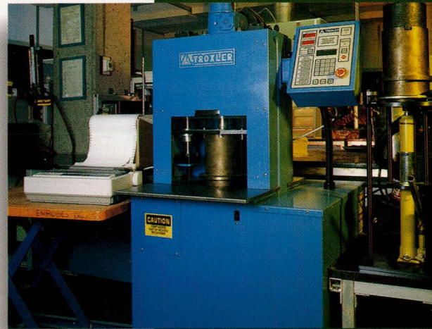
The SHRP gyratory compactor is a device used to mix-design asphalt mixes and determine their workability. (Photo: Jacques Lessard)
