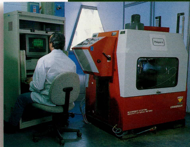
The MTQ-automated LPC rutting test machine analyzes the performance of asphalt mixes when subjected to plastic deformations such as rutting or flow under conditions resembling pavement stress. (Photo: Jacques Lessard)
