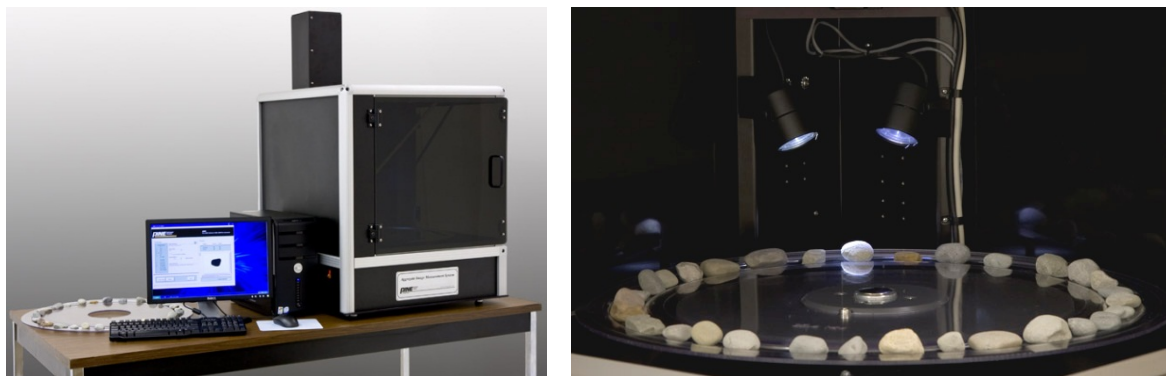
Figure 6.7: Aggregate Imaging Measurement System
