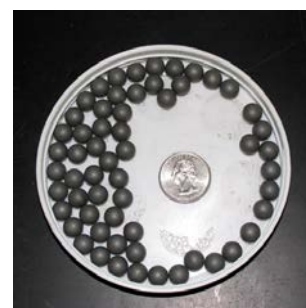
Figure 6.5: Micro–Deval apparatus and components (AASHTO/ASTM version)
