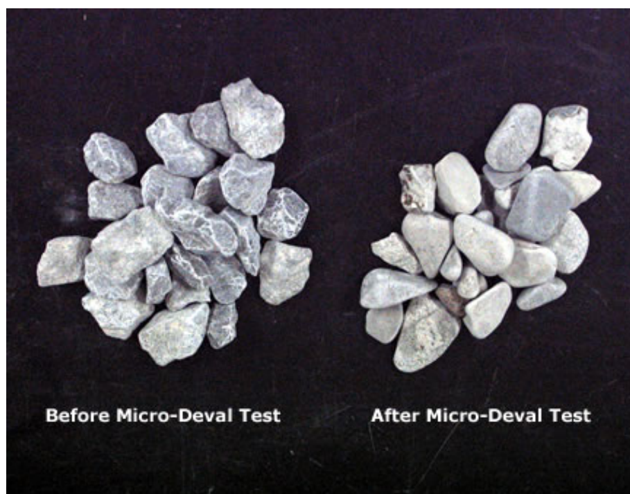
Figure 6.6: Example of aggregate stones before/after Micro-Deval test
