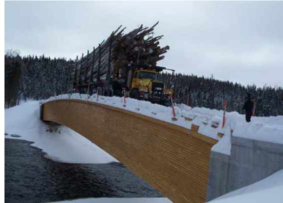
Figure 25 – Tests de chargement
