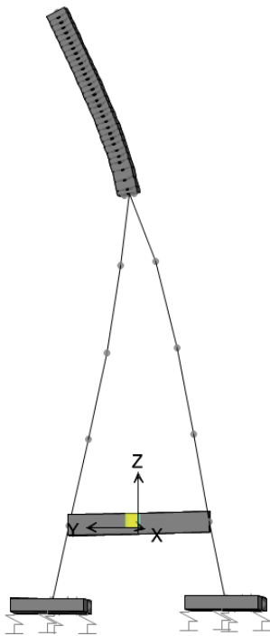
Deformed Shape (MODAL_full_bridge) - Mode 8 - T = 2.38805; f = 0.41875
