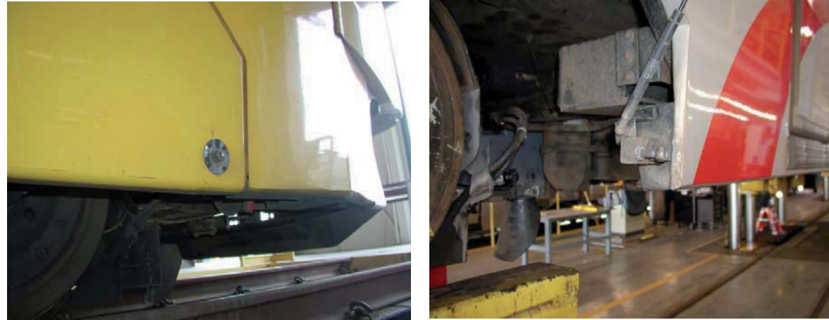
Solution: bolt modification to hold skirt shut
