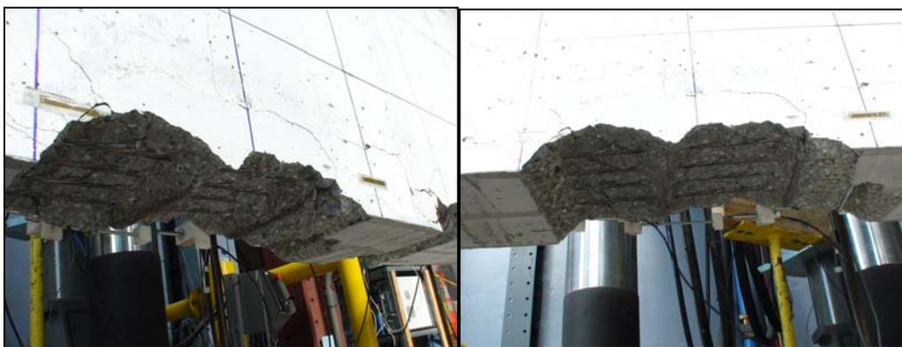
Figure 9.15 : Surface de rupture – plan de propagation de rupture – L3L
