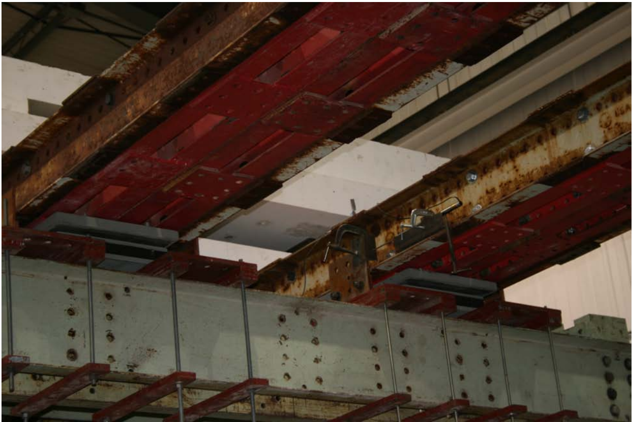
Figure 5.9: Back View Showing the Two Rollers (Slide Bearings)
