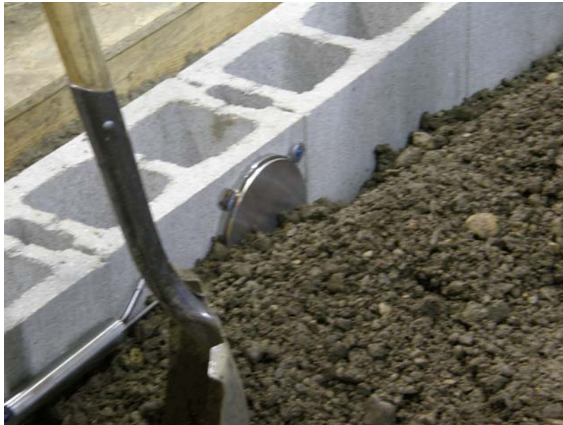
Figure 5.12: P2 Sensor Measuring Lateral Pressure at 1 st CMU Course
