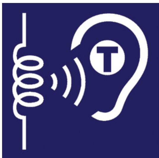
Figure A1.1 Inductive loop sign
