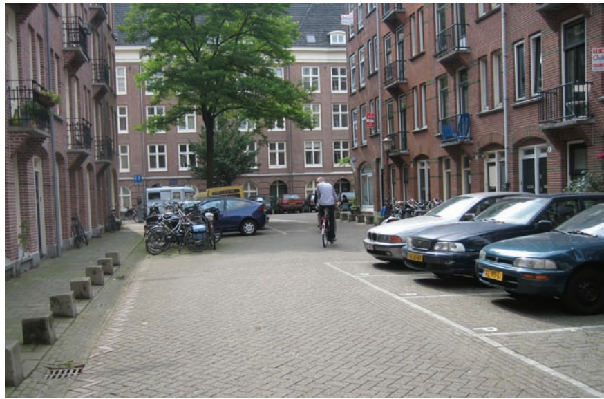
A woonerf with perpendicular parking arranged to calm the street, giving priority to pedestrians and bicyclists.
