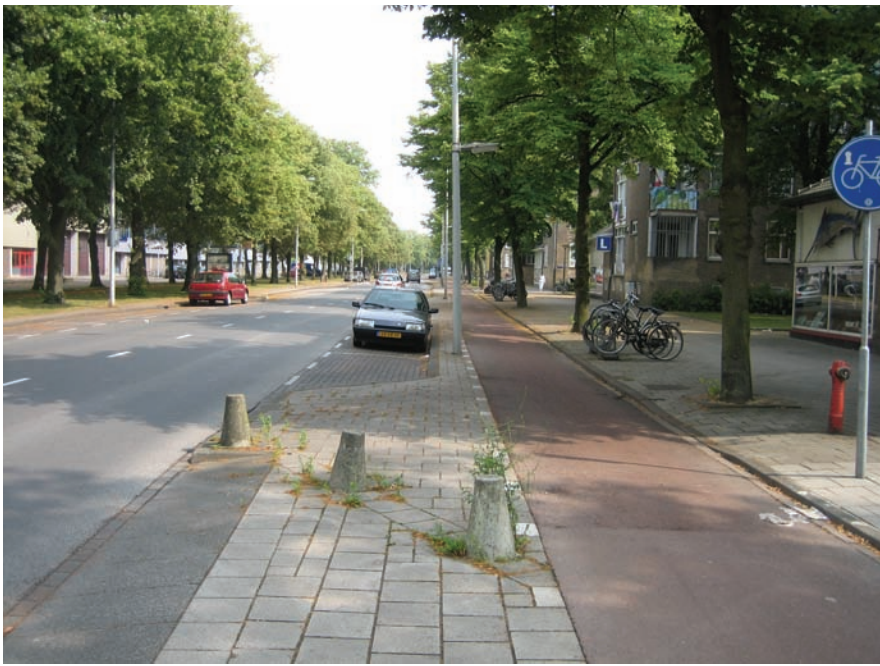
The parking lane is designed to protect the bike lane from the moving traffic lane.
