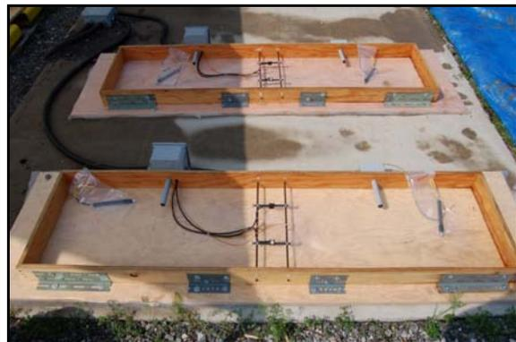
Fig. 2: Wood forms for free shrinkage slabs (slab dimensions: 2000 × 500 × 100 mm)
