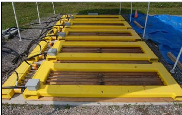
Fig. 1: Restrained shrinkage loading frames (slab dimensions: 2000 × 500 × 100 mm)
