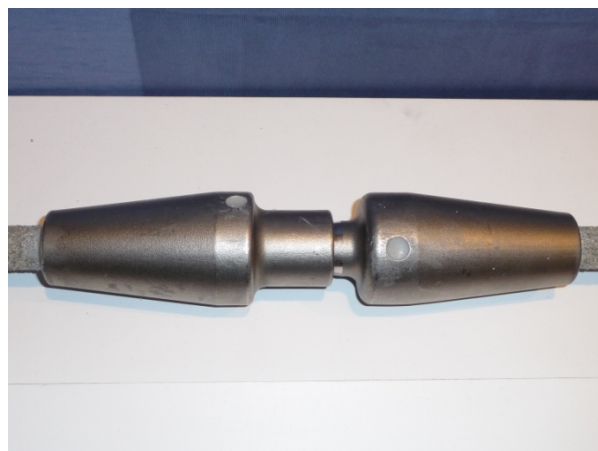
Fig. 13. 316 Stainless steel male/female connector
