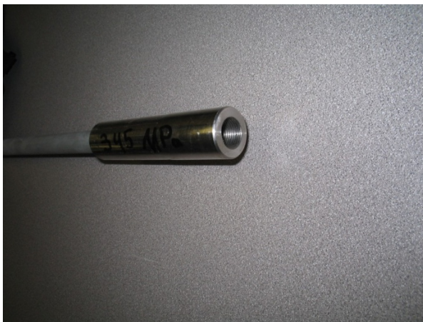
Fig. 12. Stainless steel crimped on connector
