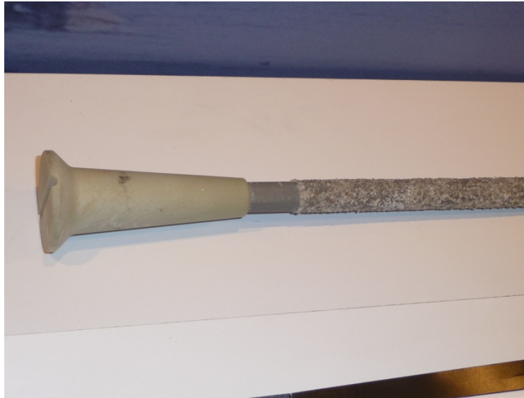
Fig. 14. Thermoplastic head secured on FRP bar
