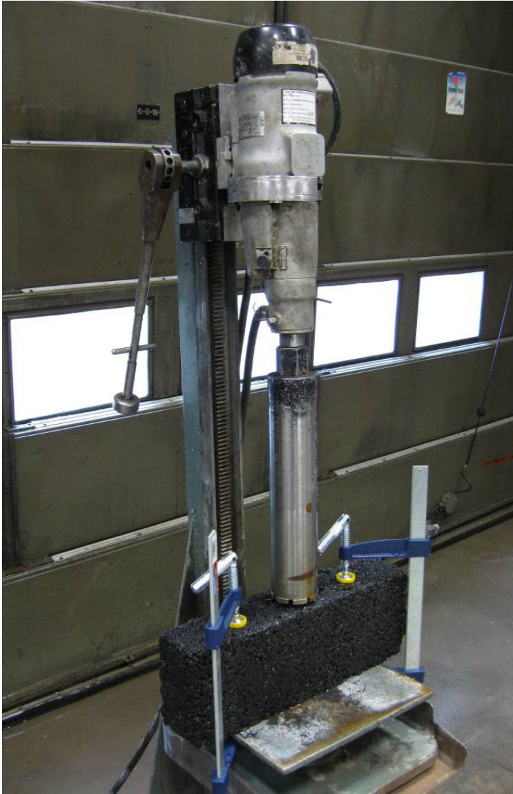
Figure 22 – Core drill for coring specimens
