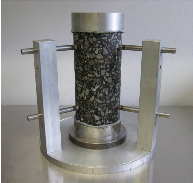
Figure 24 – Glue bench for anchor posts
