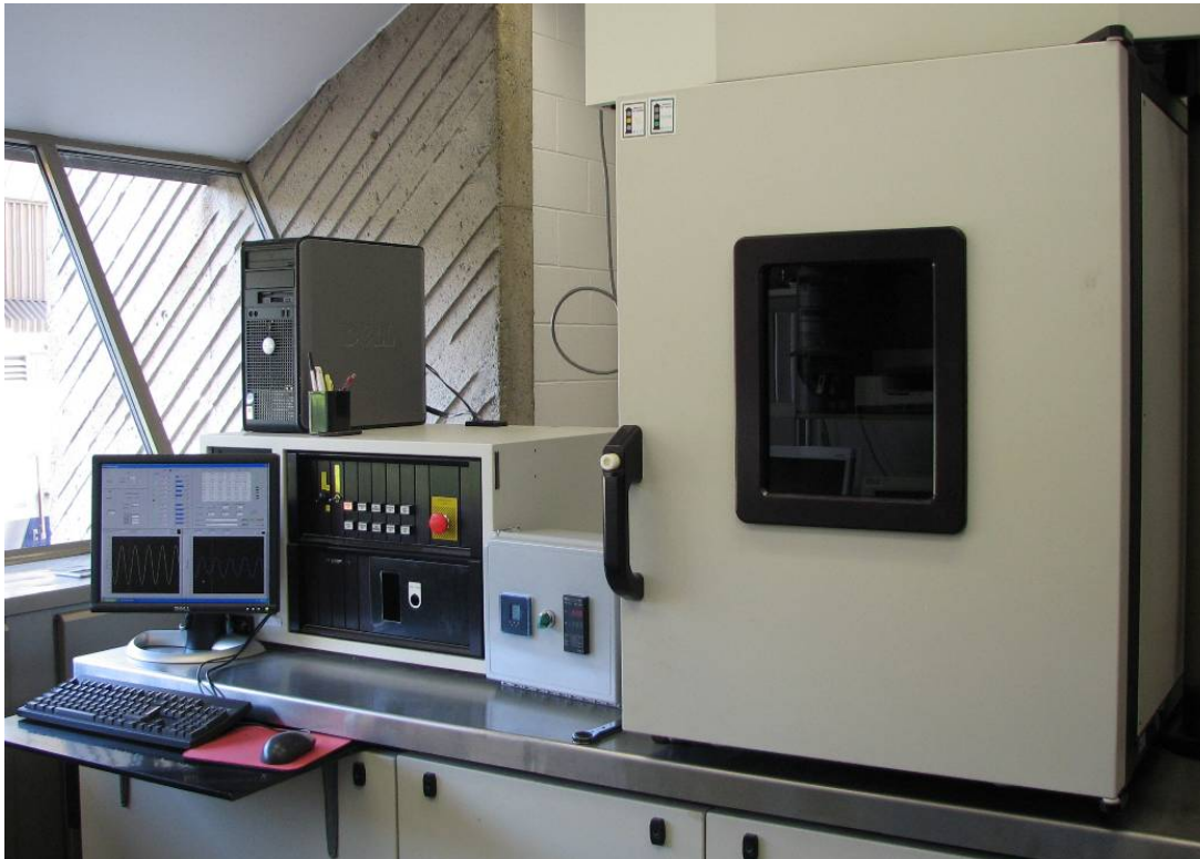
Figure 14 – Photo of the hydraulic axial testing system and controlled temperature chamber
