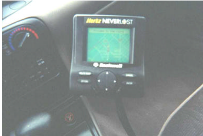
Figure 3-4: In-vehicle navigational device
