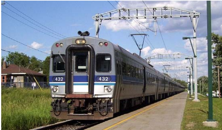
Figure 3-6 - Example of a Single-Level AC-Powered EMU, Agence Métropolitaine de Transport's Deux Montagnes Line, Montreal, Canada
