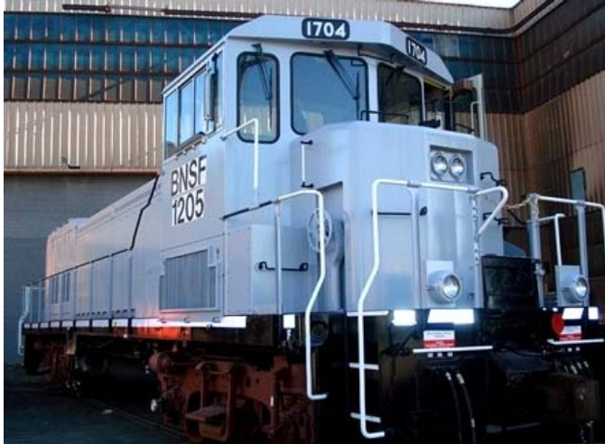
Figure 3-13 - Experimental BNSF Fuel Cell Switch Engine
