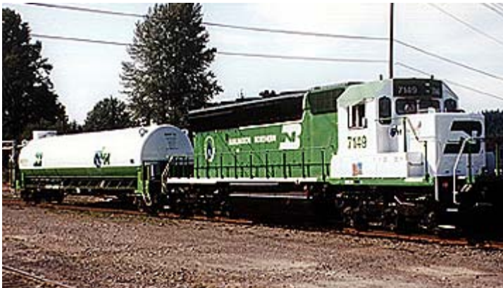
Figure 3-10 – Burlington Northern's LNG Powered Locomotive with Gas Tank
