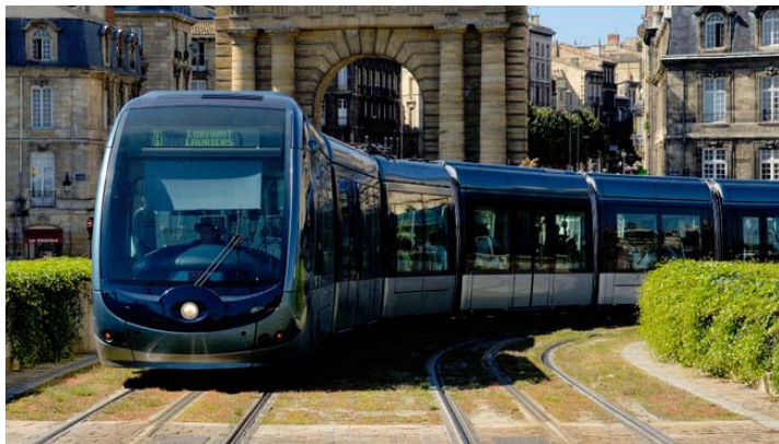
Figure 3-15 – In-Ground Power Supply System - Innorail
