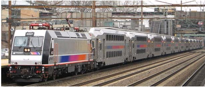
Figure 3-5 - Example of a High-Horsepower AC Electric Locomotive ALP-46
