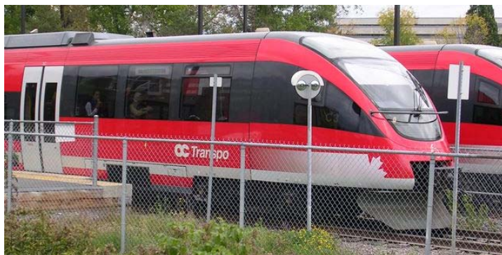
Figure 3-2 - Example of a Single-Level DMU in Ottawa, Canada
