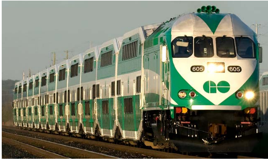
Figure 6: GO Diesel Locomotive-Hauled Train (MP40PH-3C) to be converted to Tier 4
