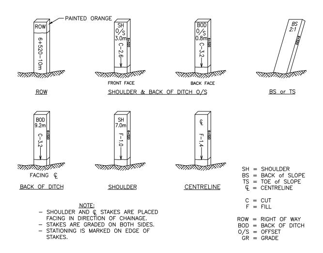
The front face of the reference stake should indicate the offset distance to the Shoulder as well as the grade.
