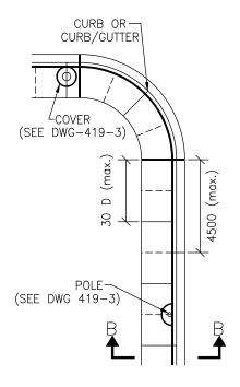
SEPARATE SIDEWALK AND CURB/GUTTER
