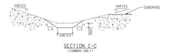
PLAN/SECTION LINES ON STANDARD DRAWING 605-3
