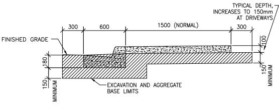
SIDEWALK WITH CURB AND GUTTER
