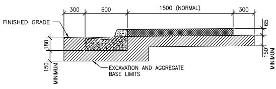
SIDEWALK WITH CURB AND GUTTER
