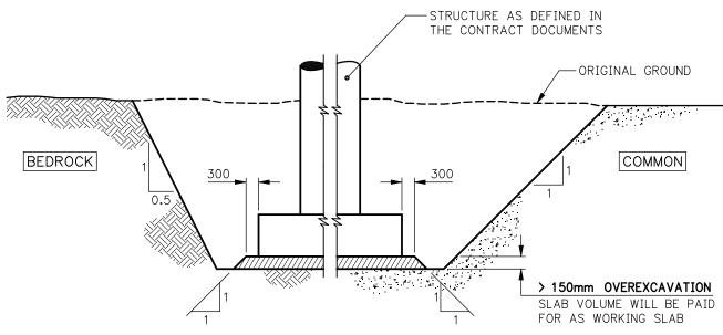
LIMITS OF WORKING SLAB CONCRETE
