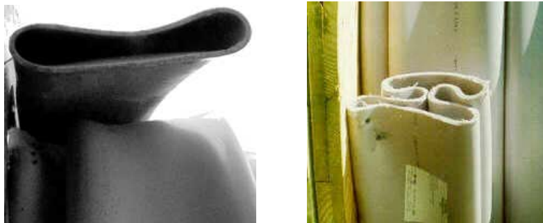
Figure 2. Ultraliner PVC Alloy Pipeliner (ranging in sizes from 4-12 in) is coiled in a flat shape and folded during insertion (left); Ultraliner PVC Alloy Pipeliners with diameters greater than or equal to 15 in are coiled in an "H" shape (right).
