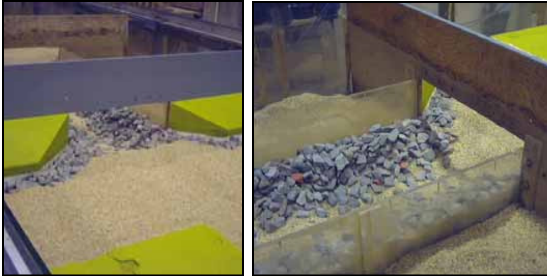
Figure 18.8. MDSHA standard plan after test (Kerenyi et al. 2007).
