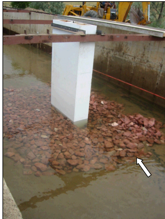
Figure 11.14. Riprap armor over geotextile containers.
