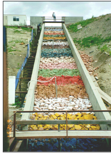
Figure 5.4. Test set up for 1997, d_{50} = 0.89 ft (271 mm).
