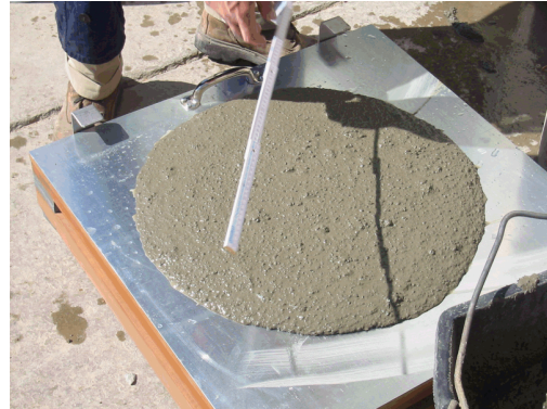
b. Measuring grout slump diameter
