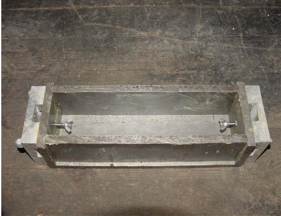
**Figure 1. Modified ASTM C157 Prism Mold**
