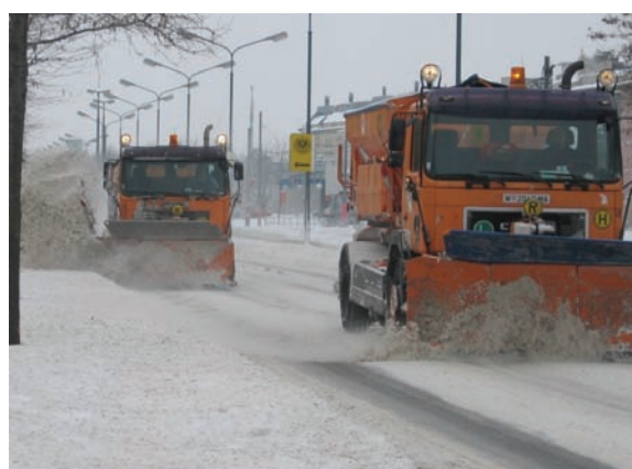
Figure 2 – Trucks with plow and F 30 equipment
