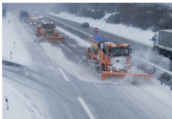
Echelon plowing with high performance winter maintenance vehicle
