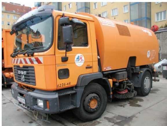
Figure 5 – Sweeping machine with sodium chloride brine spraying device
