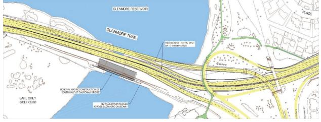
Figure 8 – Stage 3 – Remove and Construct WB Half of Causeway Bridge
