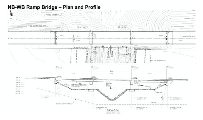
The two bridges are essentially the same in profile with the difference being shortening the west span to avoid conflicting with the West Pumphouse as illustrated below.
