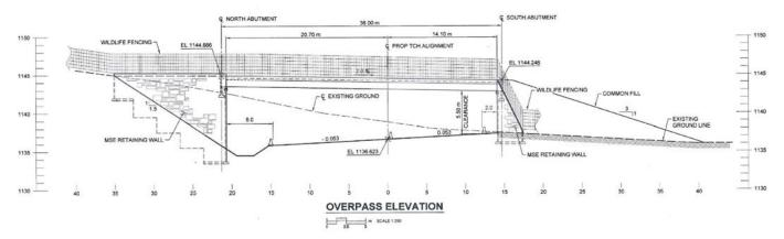
**Figure 10.** Preliminary design of Wildlife Crossing West over the Trans-Canada Highway within the Kicking Horse Canyon Project.
