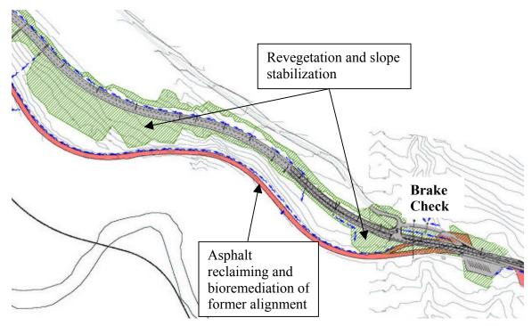
**Figure 4.** Example of planned revegetation and slope remediation proposed near Brake Check in the Kicking Horse Canyon.
