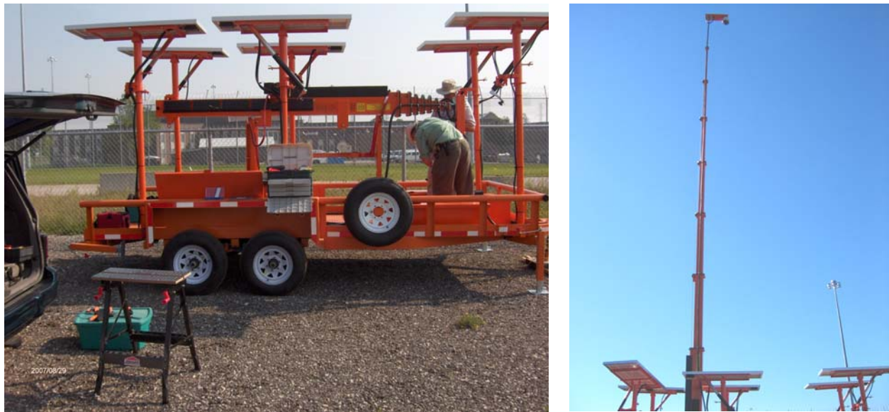
Figure 4 - Portable CCTV Trailer: in Transit Mode/with Camera Arm Extended
